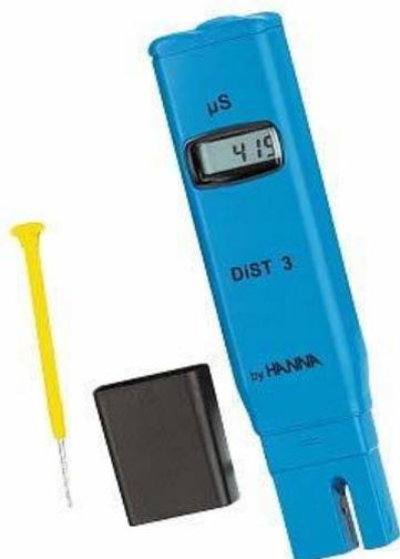
**Fig:** Conductivity meter, cover (black) and screwdriver to calibrate it.
